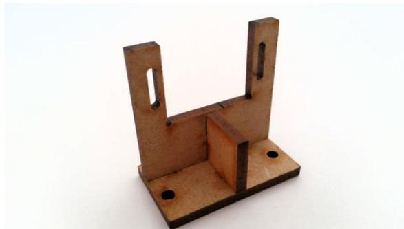
You should glue the 3 parts together, preferably with wood glue. Hobby glue and hot glue are also good. Pay attention to the partition, it only fits one way really well. Then the sides are equal. The bracket can be
